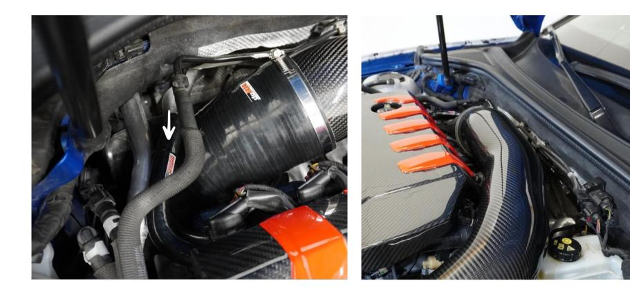
Secure the 4mm silicone vacuum hose and the crankcase hose to each other with the included stripes.
