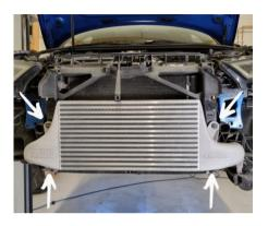
Step 17 Mount the do88 intercooler in place and tighten the OEM 4x Torx T30 screws.
