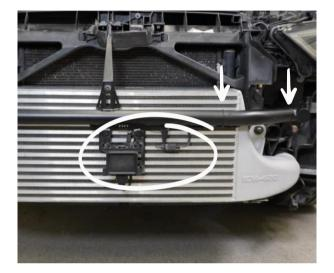
(8V only) Install the ACC and outside temperature sensor.
